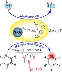
Bubbling parahydrogen gas into a solution containing a heterogeneous iridium-based catalyst (immobilized on silica supports) can produce greatly enhanced heteronuclear (e.g. <sup>15</sup>N) NMR signals when performed inside a magnetic shield prior to transfer to an NMR spectrometer for acquisition.
