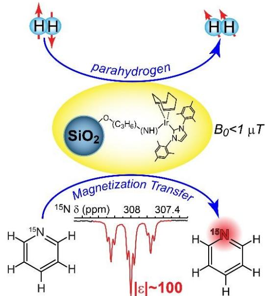
Bubbling parahydrogen gas into a solution containing a heterogeneous iridium-based catalyst (immobilized on silica supports) can produce greatly enhanced heteronuclear (e.g.  $^{15}\text{N}$ ) NMR signals when performed inside a magnetic shield prior to transfer to an NMR spectrometer for acquisition.
